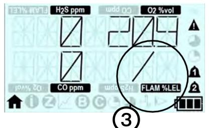
After a stabilisation time ③, if the gas level still exceeds the threshold then the sensor will be turned off and the cycle starts again.
