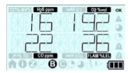
When T4 detects the applied test gas the countdown screen will be replaced with the bump test gas reading screen, this will continue to show the gas readings until the bump test result is displayed.
