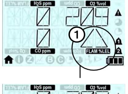
When the flammable gas exceeds the pellistor saver threshold, the detector will turn off the sensor for a minimum period of 200 seconds.
