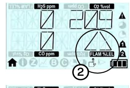
After the defined period the sensor can be re-activated by a single click of the operator button ② once the instrument is in a clean air environment.v
