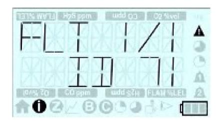
In addition the Information screen will also display any identified fault; this fault will be indicated by a warning icon on the home screen.
