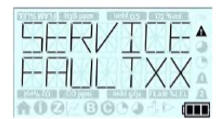
If T4 detects an internal fault that requires T4 to be returned for servicing 'Service' message as shown will be displayed on the screen, where 'XX' represents a specific fault ID code.
