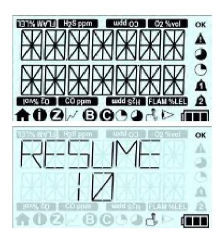
Firstly a test screen will be displayed showing all the possible LCD segments and icons turned on.
