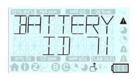
T4 will indicate a low battery alarm when the battery has a maximum of 30 minutes remaining life.
